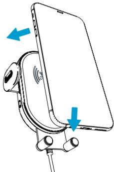
NOTE: if the Type-C cable is not connected to the charger, the clamps will not close automatically. You will need to press the lateral button to close the clamps around your phone. When the power is off, it will beep 5 times to remind you to take away the phone.
