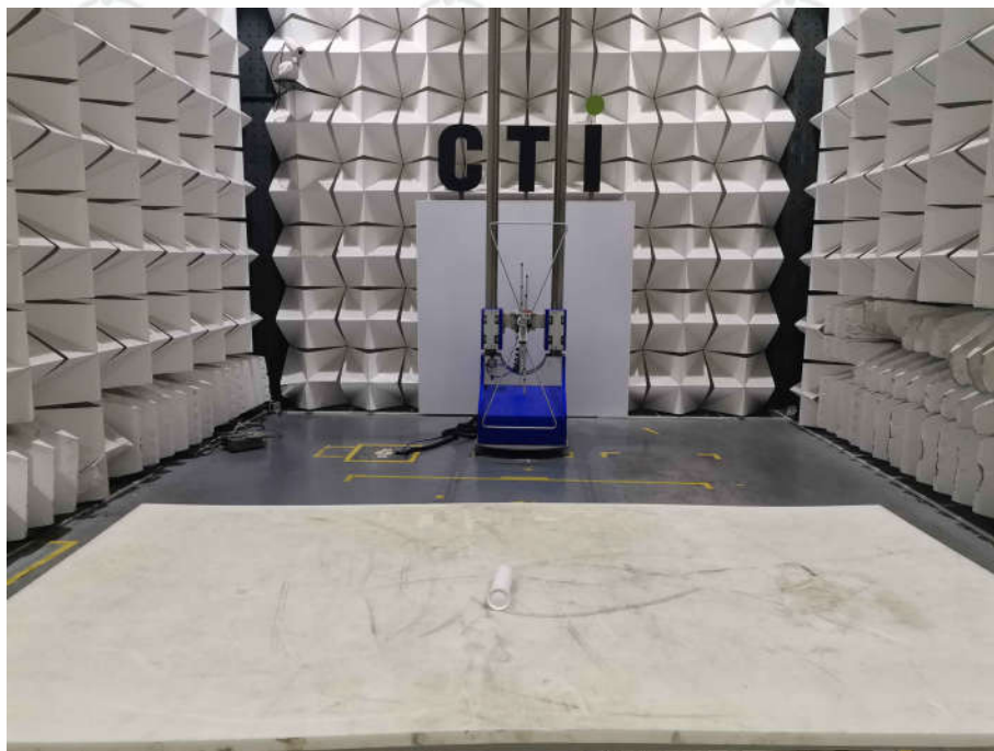
Radiated spurious emission Test Setup-1(Below 1GHz)
