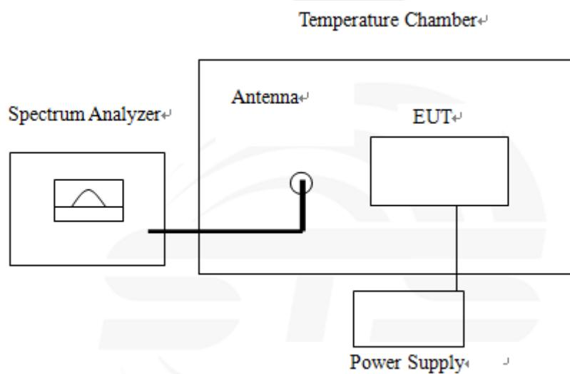
The EUT which is powered by the Battery, is coupled to the Spectrum Analyzer; the RF load attached to the EUT antenna terminal is 50Ohm; the path loss as the factor is calibrated to correct the reading.
