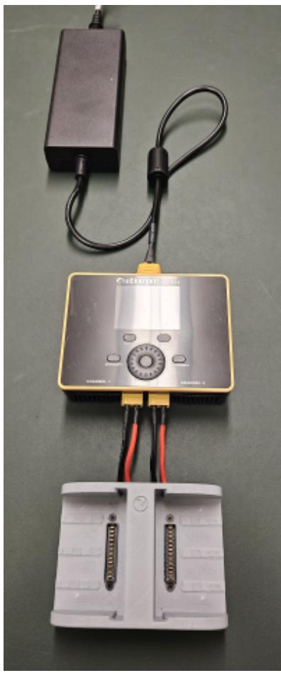
Connect the AD/DC adapter to the DX8 charger using the XT90 connector on the back of the charger.
