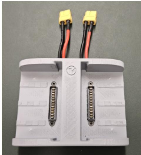
Battery dock for two flight batteries with XT60 connectors to connect to DX8 charger
