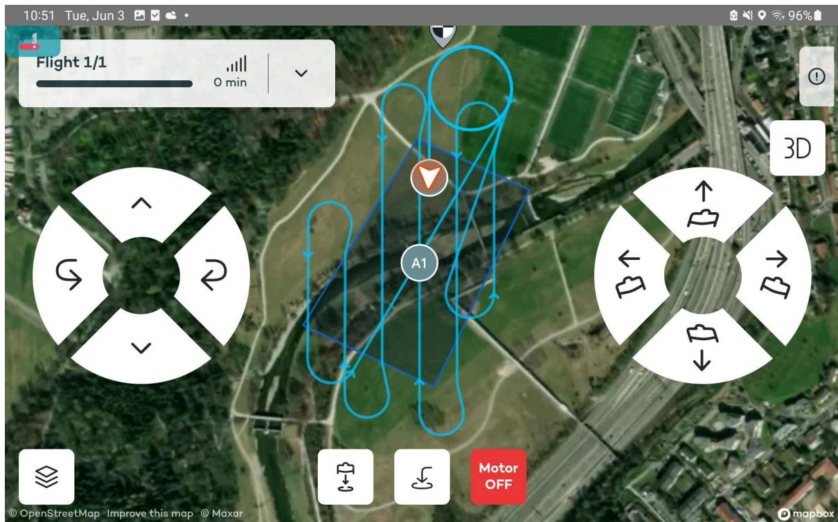
With the left-side buttons, you can command WingtraRay to move up and down or control the orientation along its axis.
