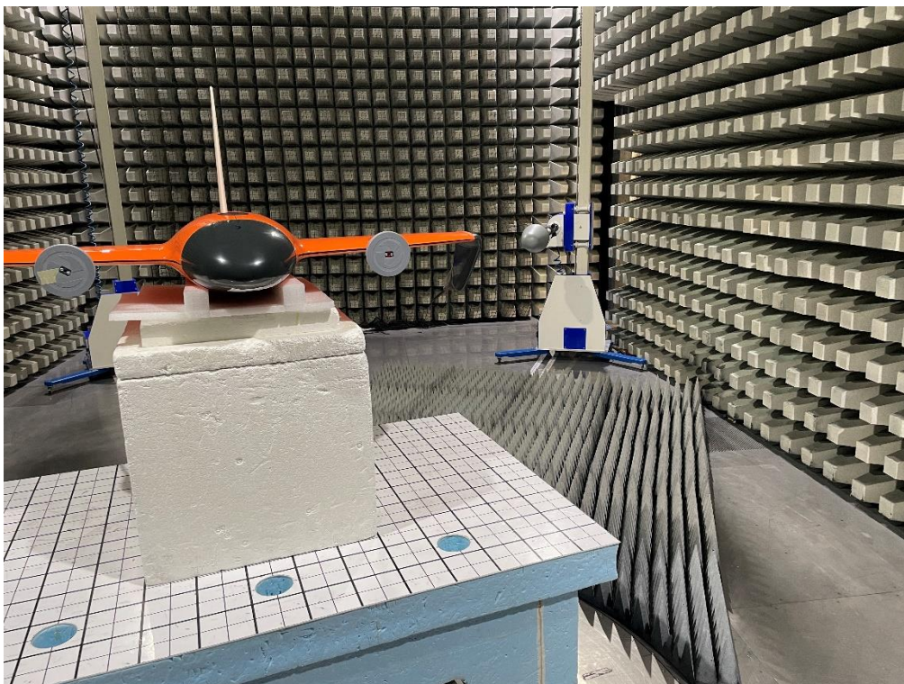
Photo 6 Radiated Test Setup 1 - 18 GHz
