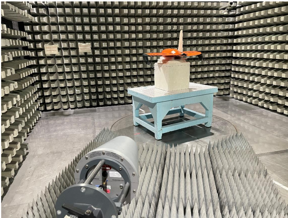
Photo 5 Radiated Test Setup 1 - 18 GHz
