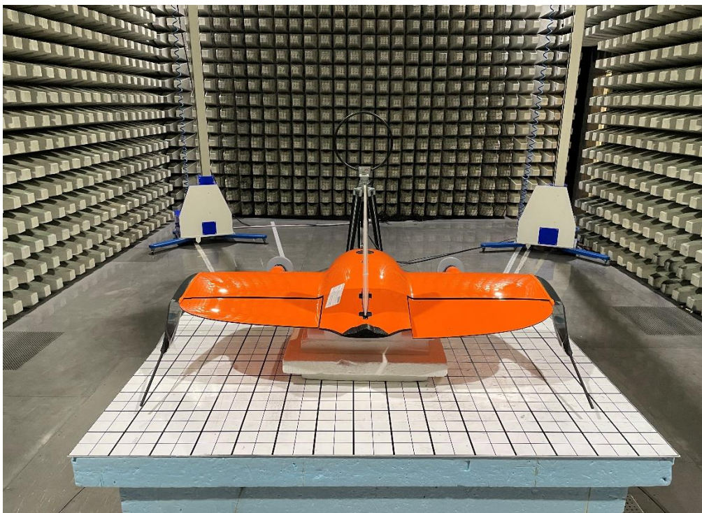
Photo 2 Radiated Test Setup below 30 MHz
