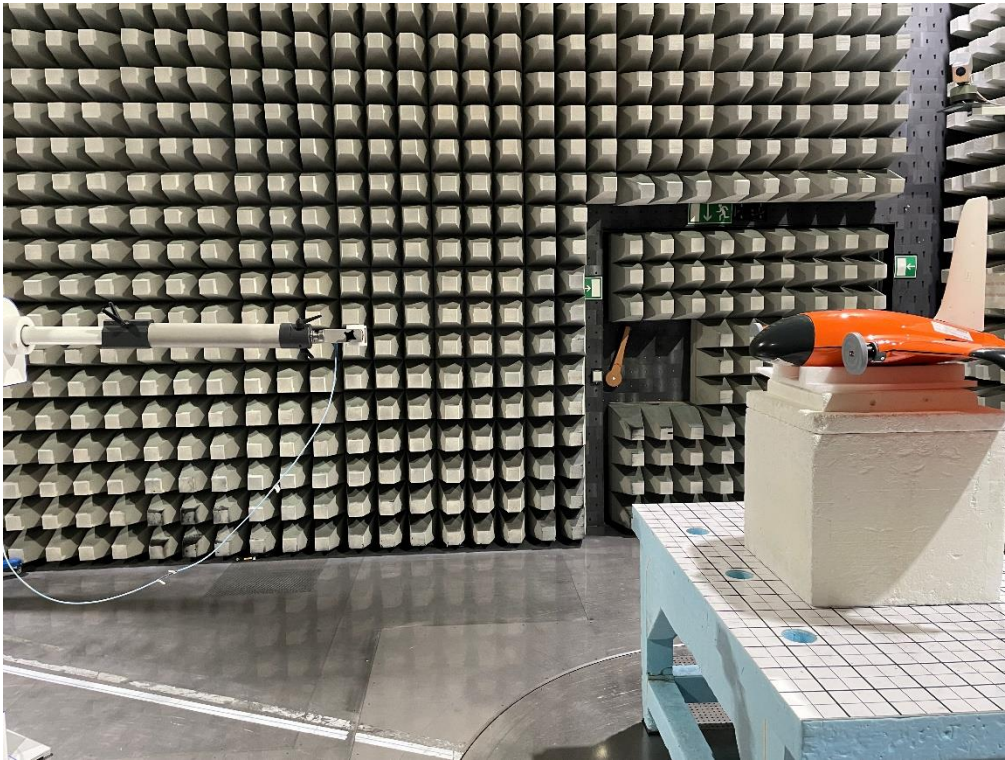
Photo 7 Radiated Test Setup 18-40 GHz
