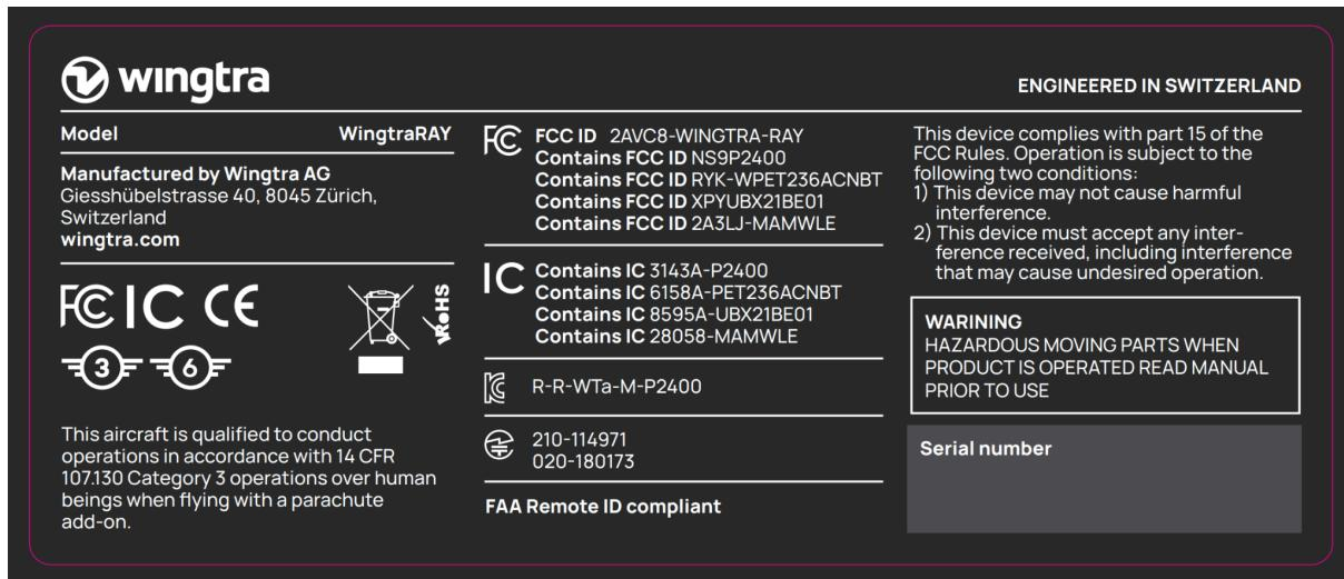
The label is placed inside the WingtraRay payload bay as shown in the picture below. The label size is 120 x 50 mm and it is secured using a permanent adhesive applied on its full back surface.
