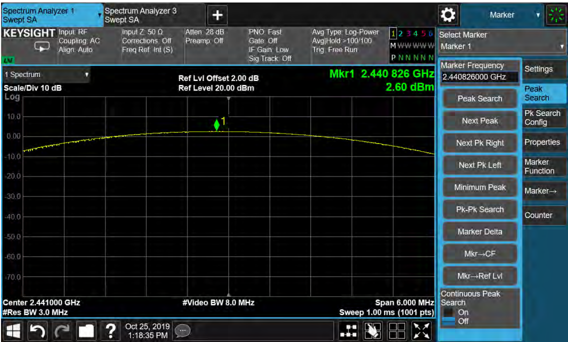
Figure 8: Maximum Conducted Output Power, 2441MHz, 8-DPSK
