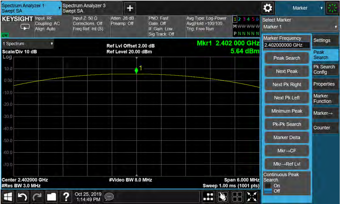
Figure 1: Maximum Conducted Output Power, 2402MHz, GFSK
