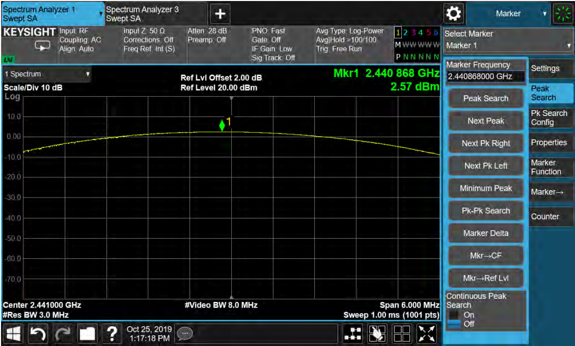
Figure 5: Maximum Conducted Output Power, 2441MHz, \pi/4 -DQPSK
