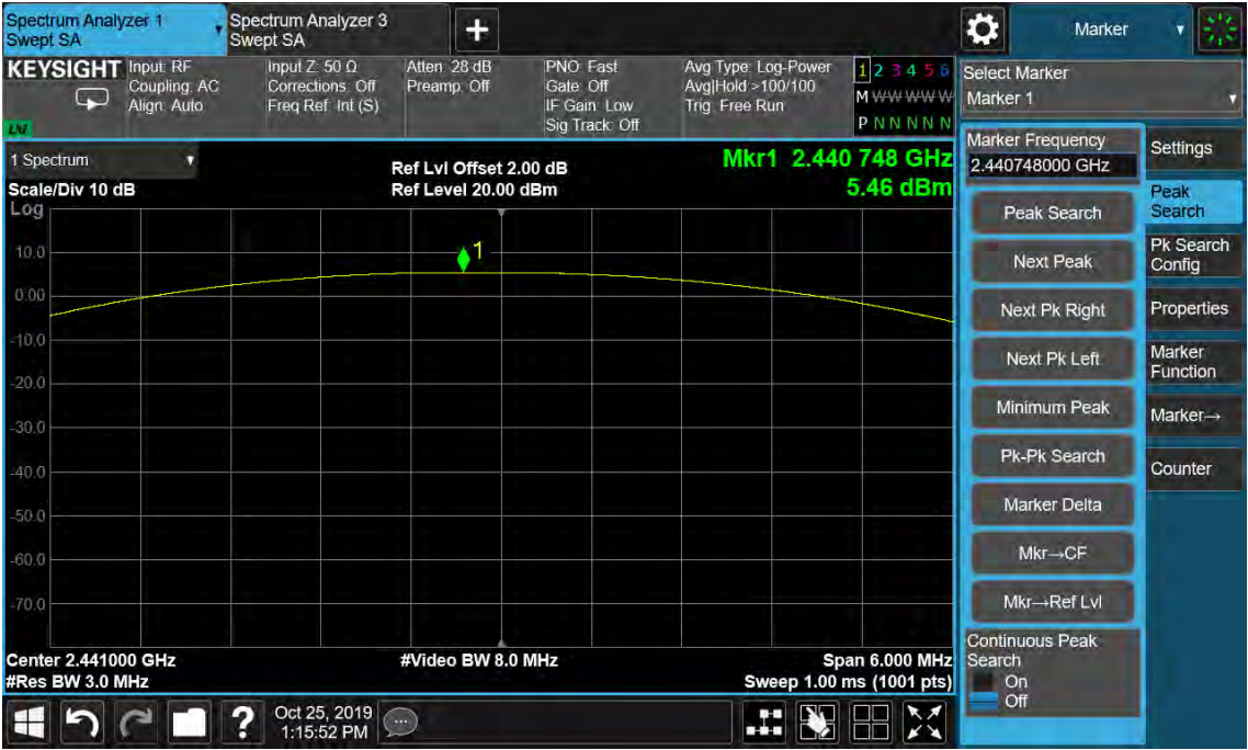
Figure 2: Maximum Conducted Output Power, 2441MHz, GFSK
