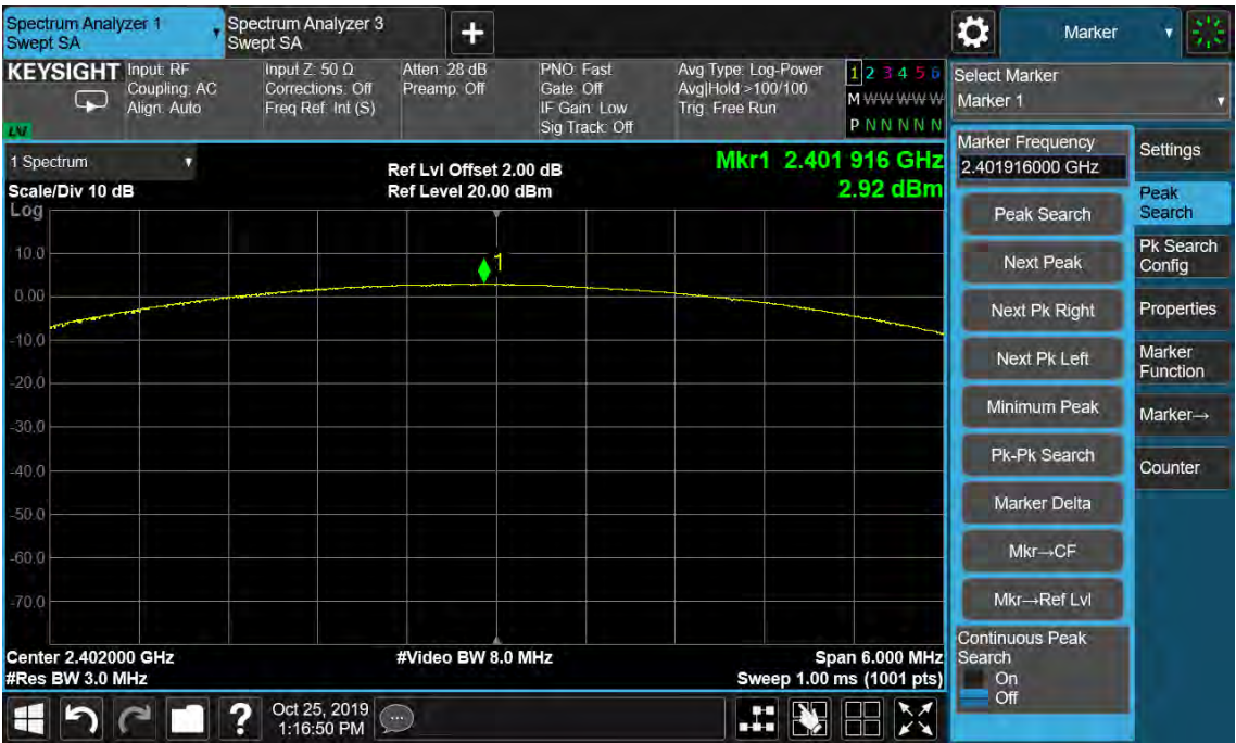
Figure 4: Maximum Conducted Output Power, 2402MHz, \pi/4 -DQPSK
