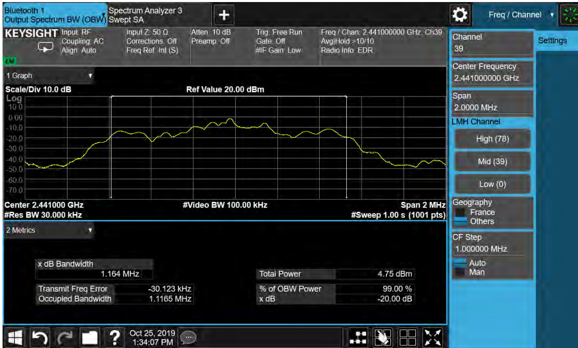
Figure 14: 20dB Bandwidth and 99% Bandwidth, 2441MHz, 8-DPSK
