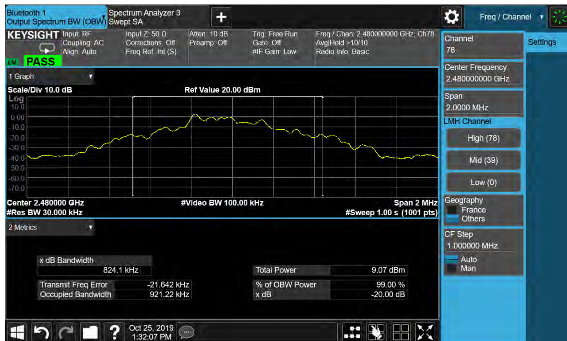
Figure 12: 20dB Bandwidth and 99% Bandwidth, 2480MHz, GFSK
