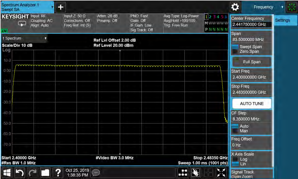
Figure 26: Number of Hopping Frequency, Hopping Mode, GFSK
