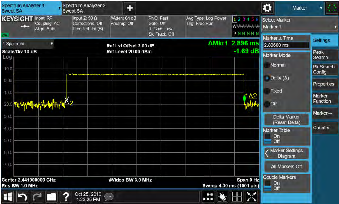
Figure 30: Time of Occupancy, 2441MHz, GFSK DH5
