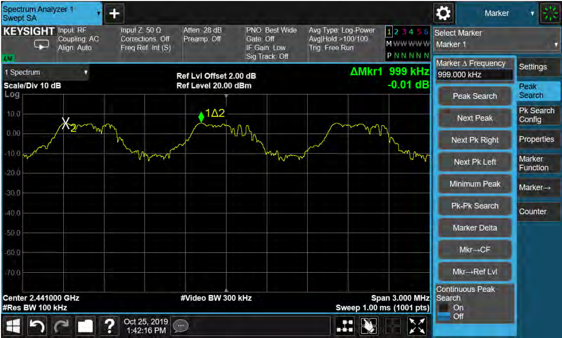
Figure 24: Hopping Frequency Separation, Hopping Mode, GFSK
