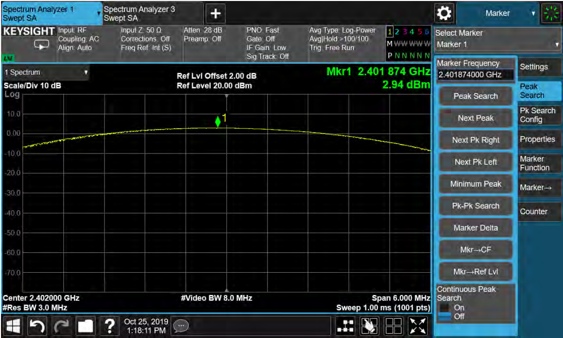
Figure 7: Maximum Conducted Output Power, 2402MHz, 8-DPSK
