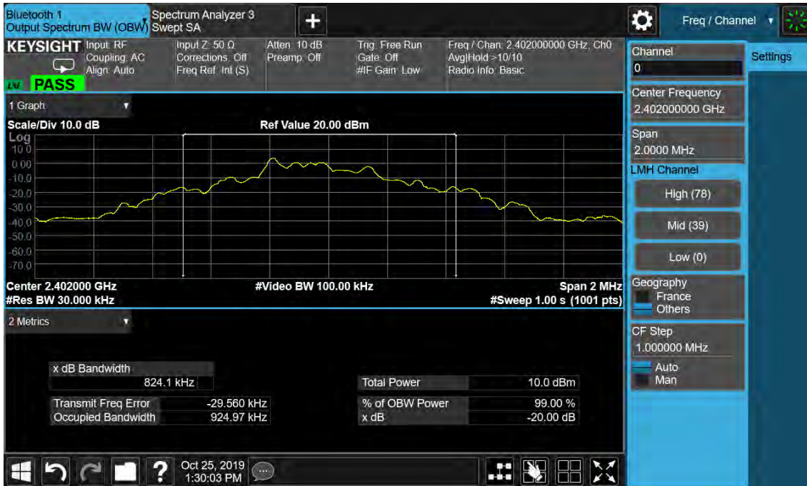
Figure 10: 20dB Bandwidth and 99% Bandwidth, 2402MHz, GFSK
