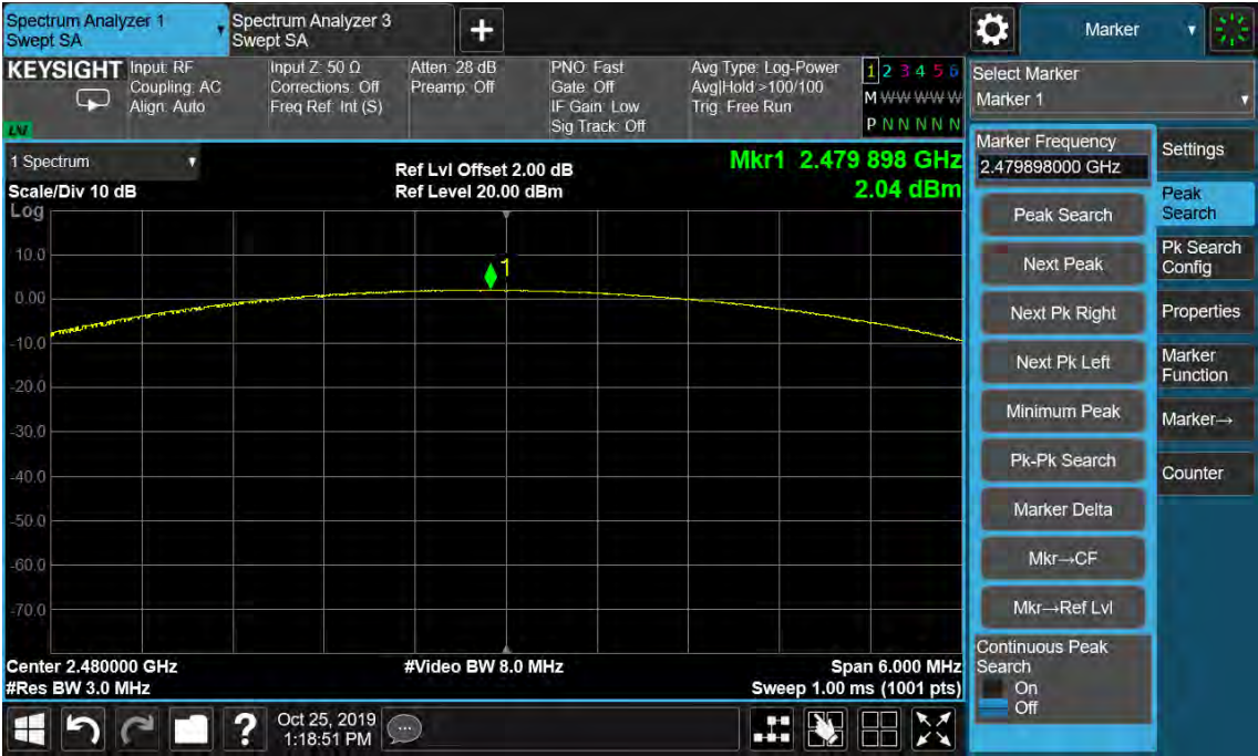
Figure 9: Maximum Conducted Output Power, 2480MHz, 8-DPSK
