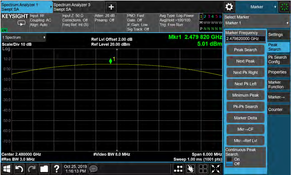
Figure 3: Maximum Conducted Output Power, 2480MHz, GFSK
