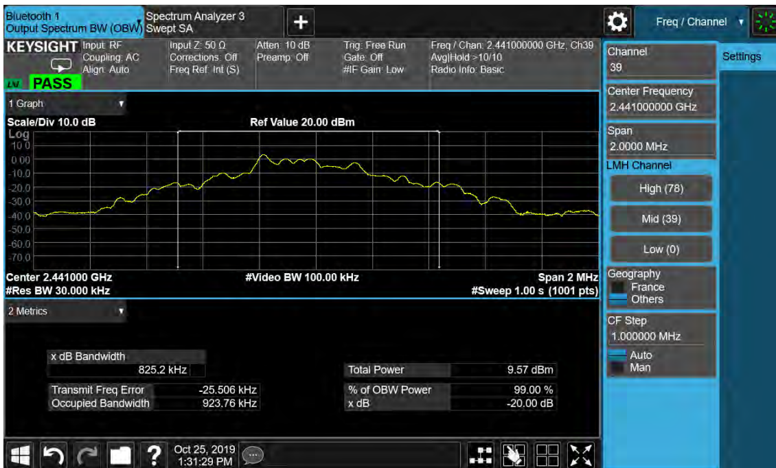
Figure 11: 20dB Bandwidth and 99% Bandwidth, 2441MHz, GFSK
