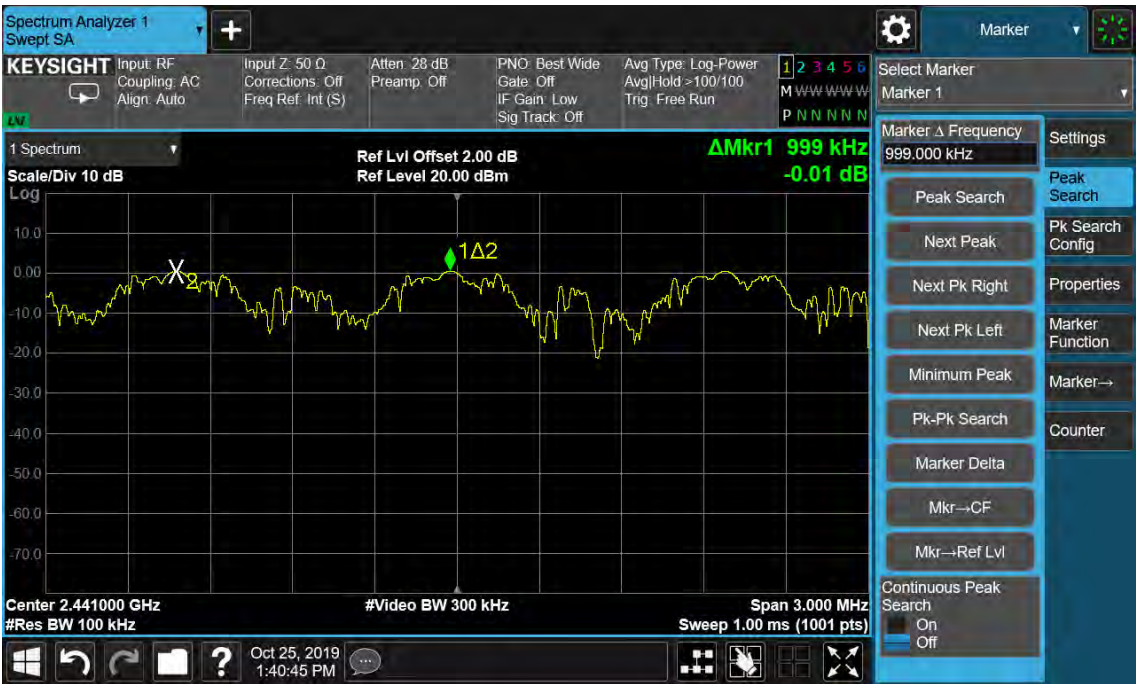
Figure 25: Hopping Frequency Separation, Hopping Mode, 8DPSK
