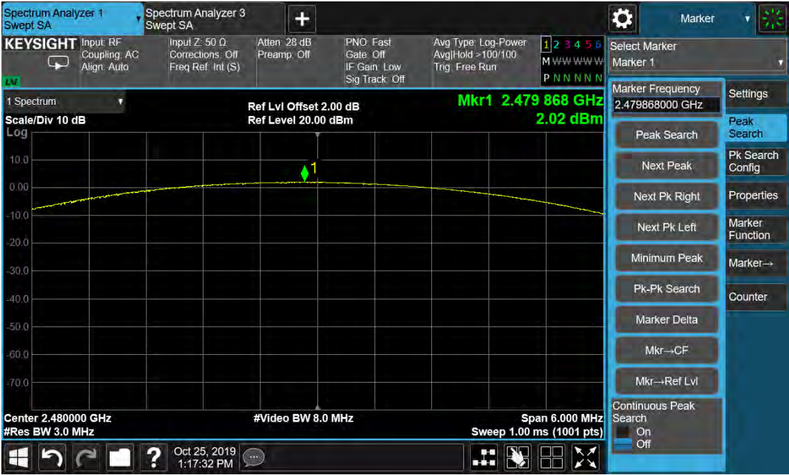
Figure 6: Maximum Conducted Output Power, 2480MHz, \pi/4 -DQPSK
