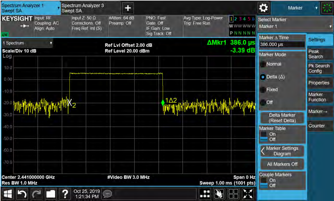
Figure 28: Time of Occupancy, 2441MHz, GFSK DH1
