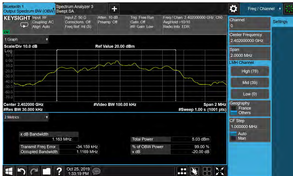
Figure 13: 20dB Bandwidth and 99% Bandwidth, 2402MHz, 8-DPSK
