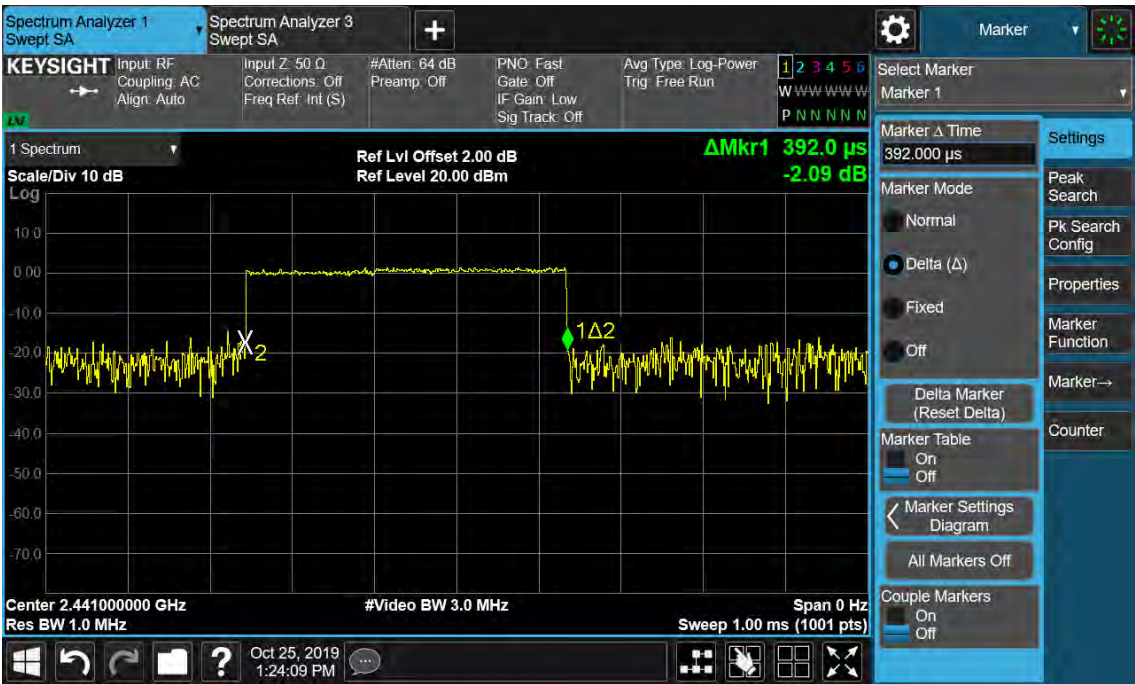
Figure 31: Time of Occupancy, 2441MHz, 8-DPSK DH1
