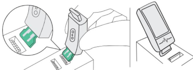
**3** Remove device from the power supply once fully charged.
