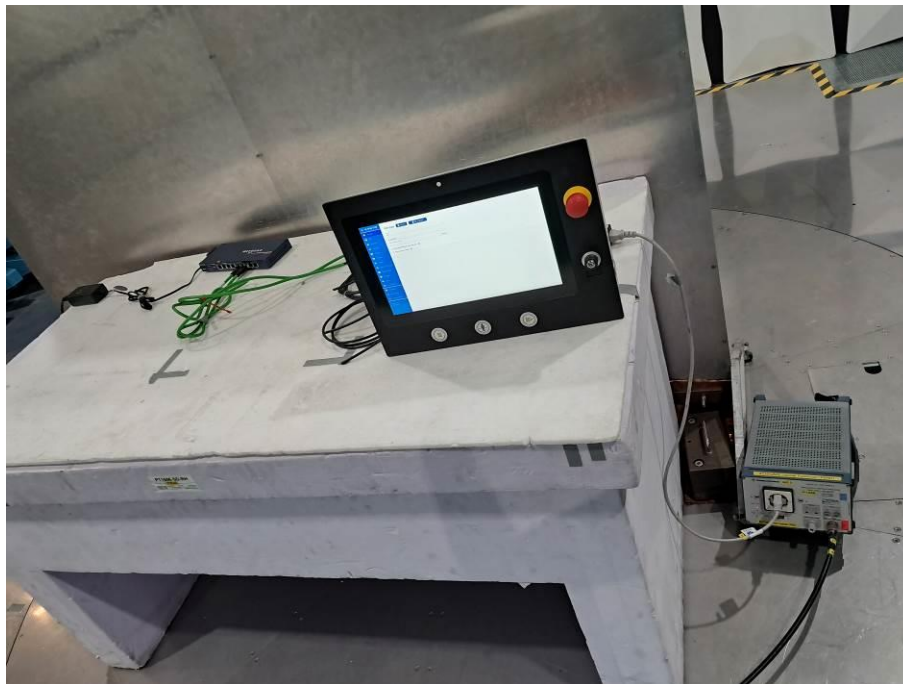
Figure 6-1: test setup Low voltage AC mains continuous disturbance
