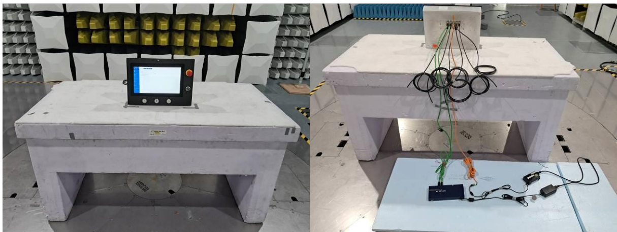
Figure 6-6: test setup for radiated disturbances 1 GHz to 18 GHz
