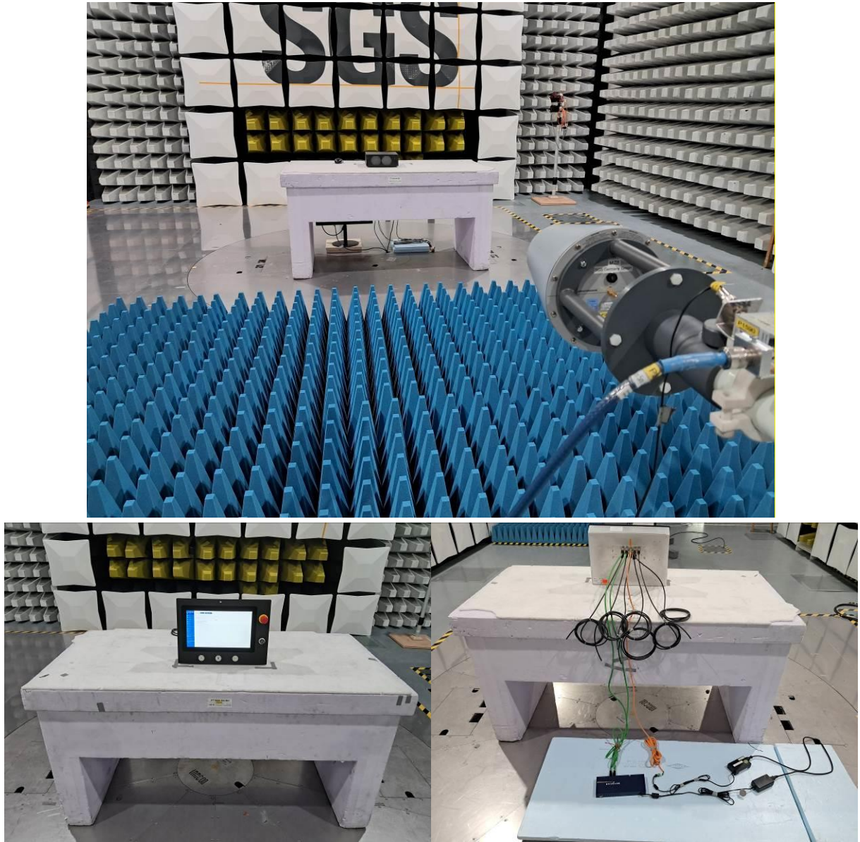
Figure 6-6: test setup for radiated disturbances 1 GHz to 18 GHz
