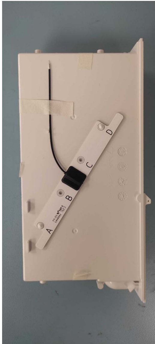
Figure 8: Example of 21173 PCB Dipole installed with heat-stake in the sachet bin area.
