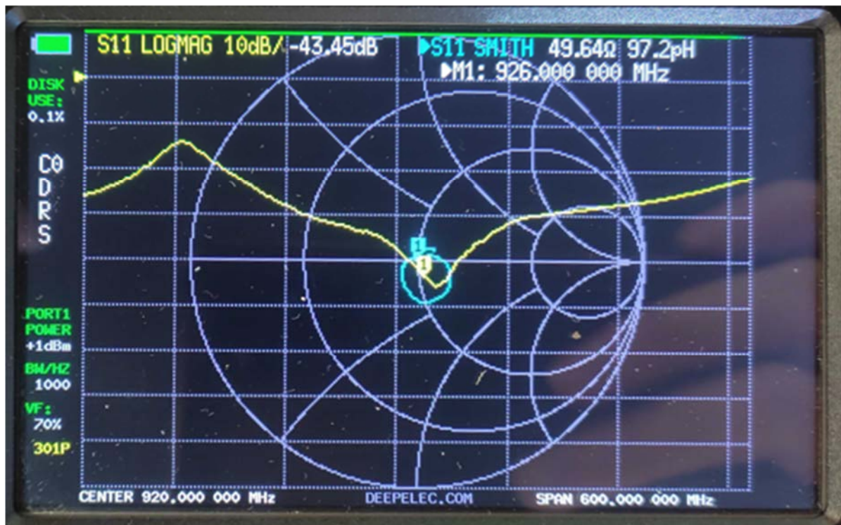
Figure 1: Antenna on VNA, Centerpoint is 926MHz
