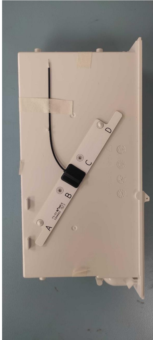
Figure 6: Example of 21173 installed with heat-stake in the sachet bin area.
