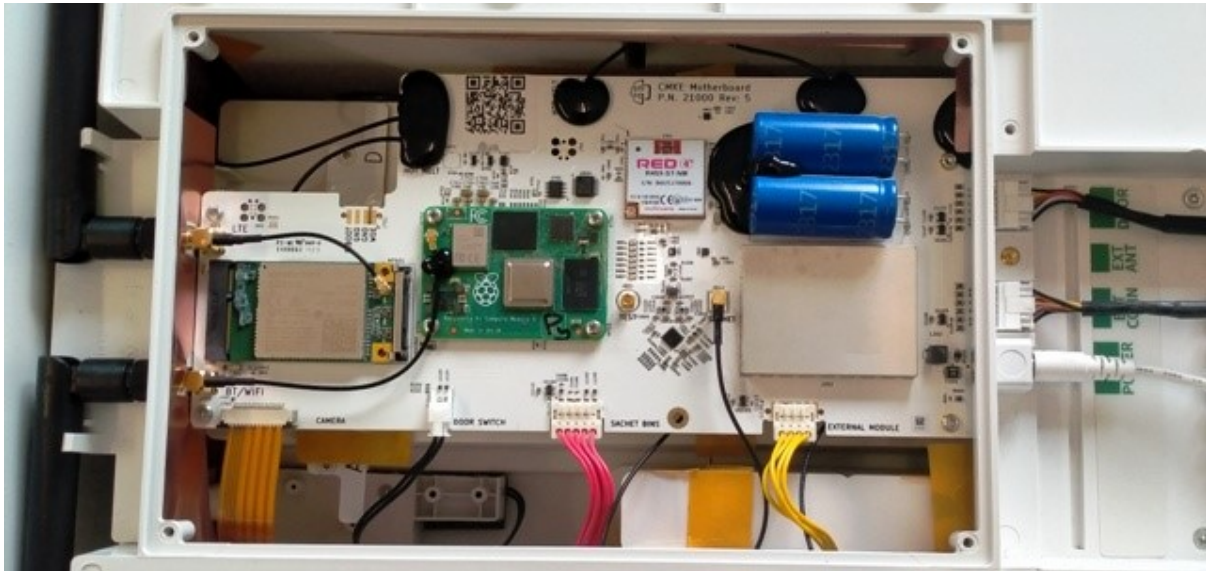
Main Circuit Board showing RED, Raspberry Pi and EG21 Cellular Module
