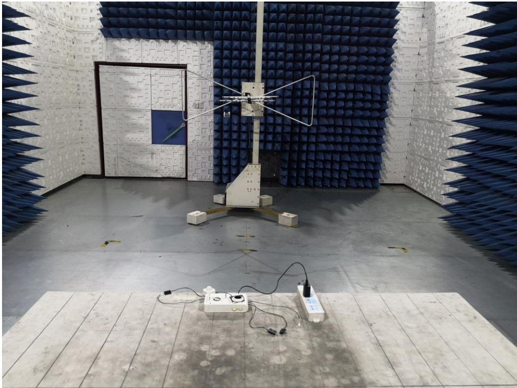
FCC RADIATED EMISSION TEST SETUP ABOVE 1GHZ
