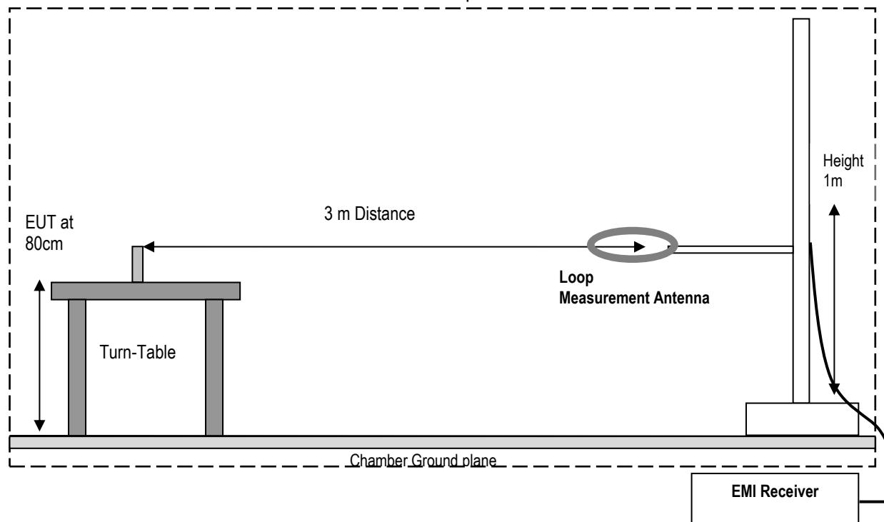
**Radiated Emissions Test Setup 30MHz-1GHz Measurements**
