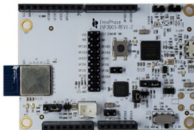
INP3014 (Includes INP1014 module with PCB Antenna)
