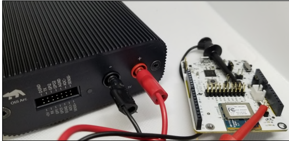
Figure 14: Current measurement setup using Otti Arc
