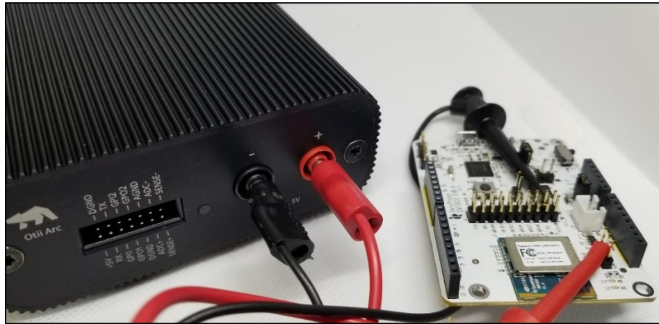
Figure 15: Current measurement setup using Otti Arc
