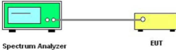
The EUT which is powered by the Battery, is connected to the Spectrum Analyzer; the RF load attached to the EUT antenna terminal is 50Ohm; the path loss as the factor is calibrated to correct the reading.
