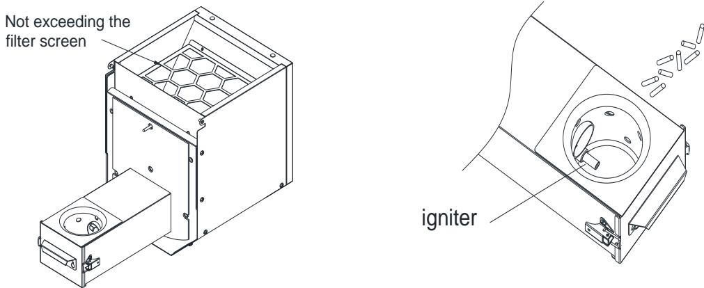
The device starts to ignite. White smoke will be emitted during the ignition of the fuel, and personnel can stay away from the operating equipment after waiting for the ignition to complete.
