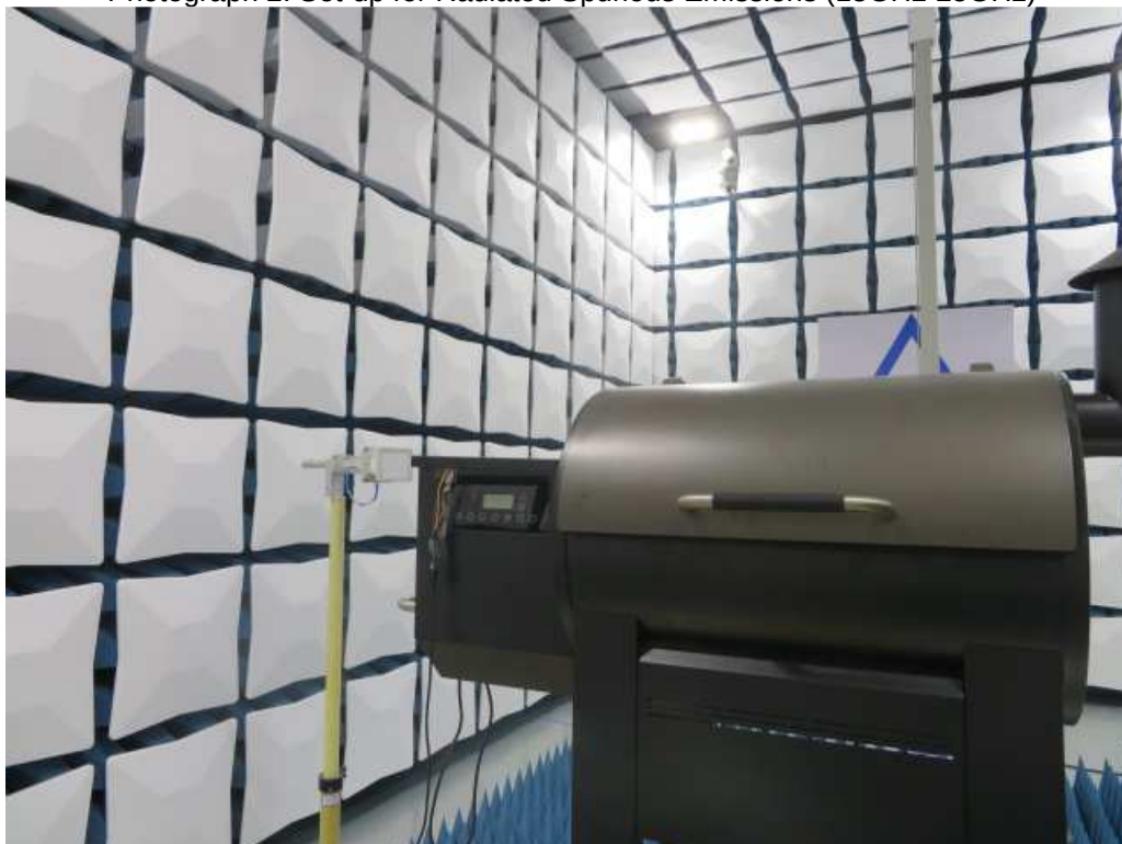
Photograph 2: Set-up for Radiated Spurious Emissions (18GHz-25GHz)
