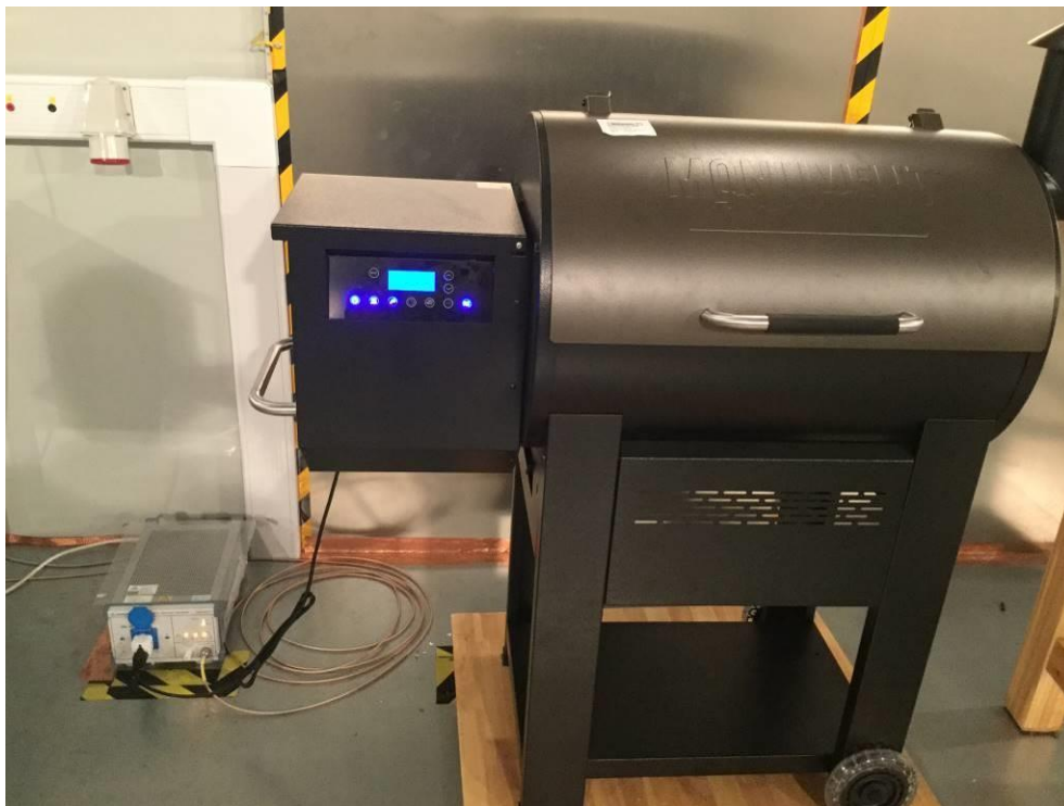
Photograph 2: Set-up for Conducted Emission on AC Mains
