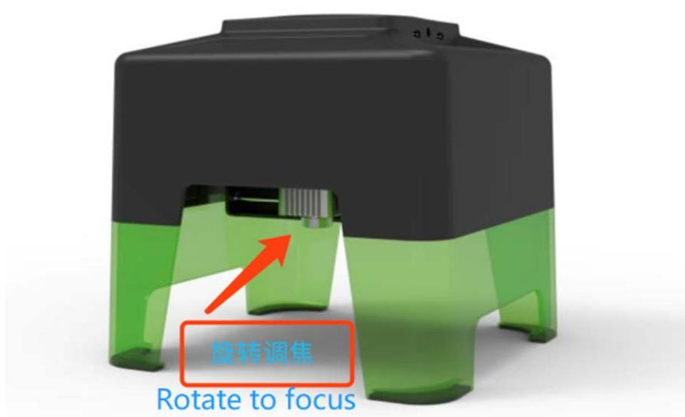
Observe the ray of light fall to the smallest point on the surface of the object. When the light is rotated to the smallest point, the focal length is adjusted. Note that the smaller the focus adjustment, the more delicate the effect of image tuning, if the focal length is not adjusted well, there may be no engraved image.
