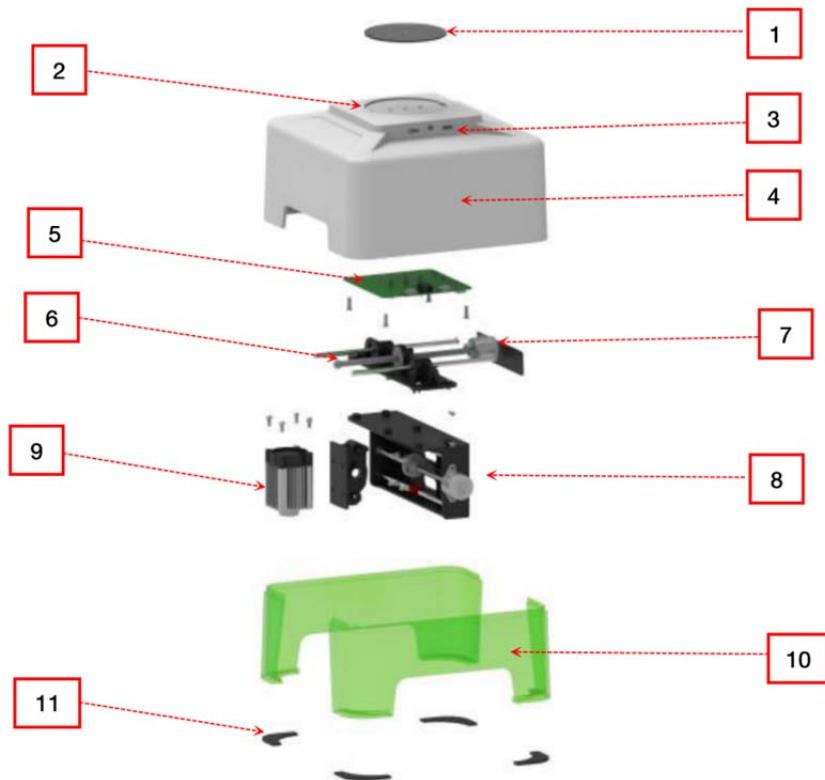
① indicator light panel ② indicator light ③ external interface ④ shell ⑤ main control circuit board ⑥ Y axis screw rod ⑦ motor ⑧ X axis screw rod ⑨ laser tube ⑩ Eye protector stents ⑪ rubber foot
