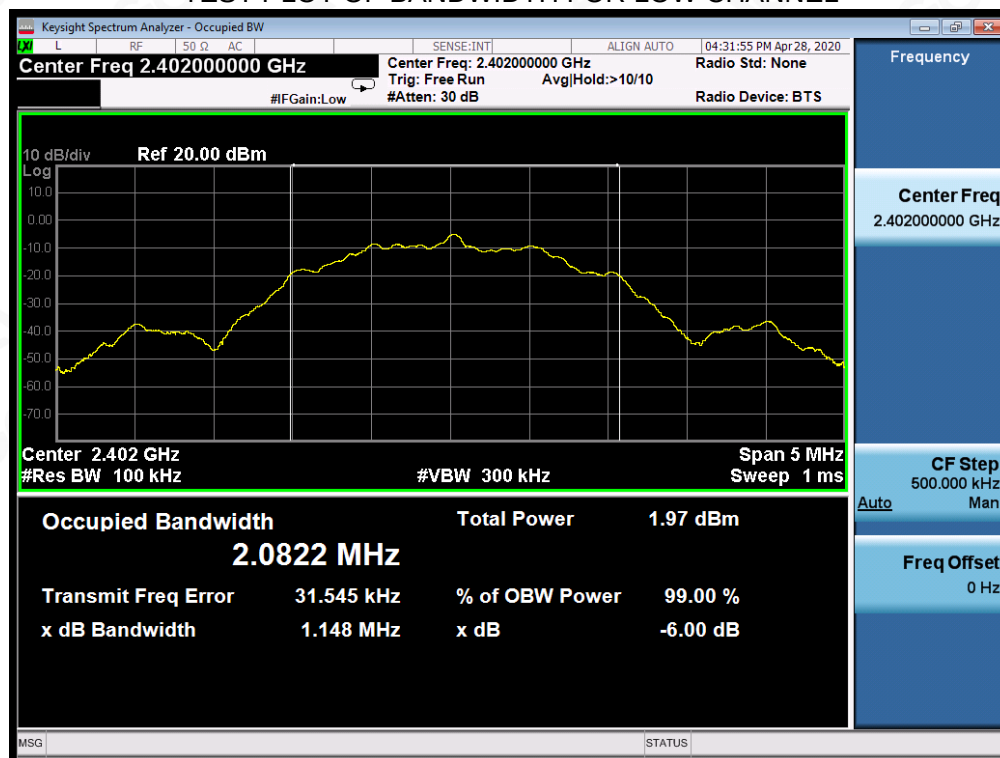
TEST PLOT OF BANDWIDTH FOR LOW CHANNEL
