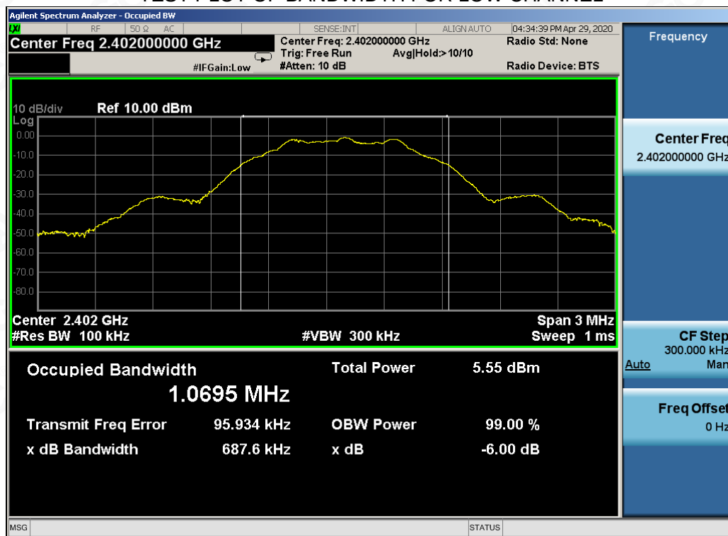
TEST PLOT OF BANDWIDTH FOR LOW CHANNEL
