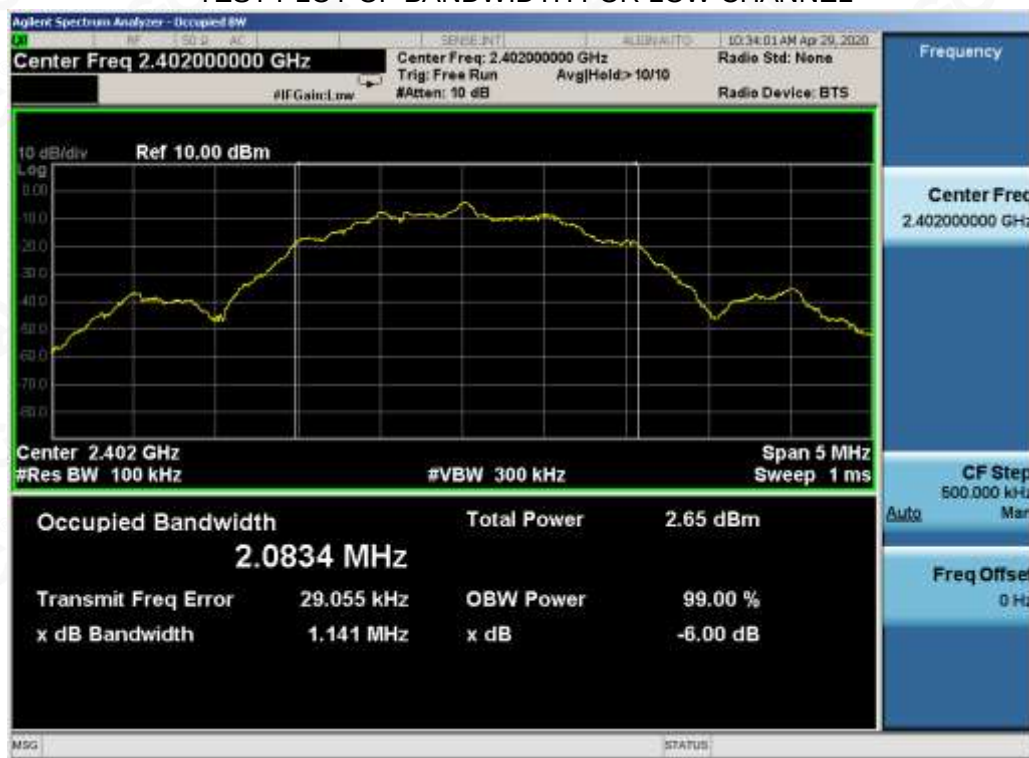
TEST PLOT OF BANDWIDTH FOR LOW CHANNEL
