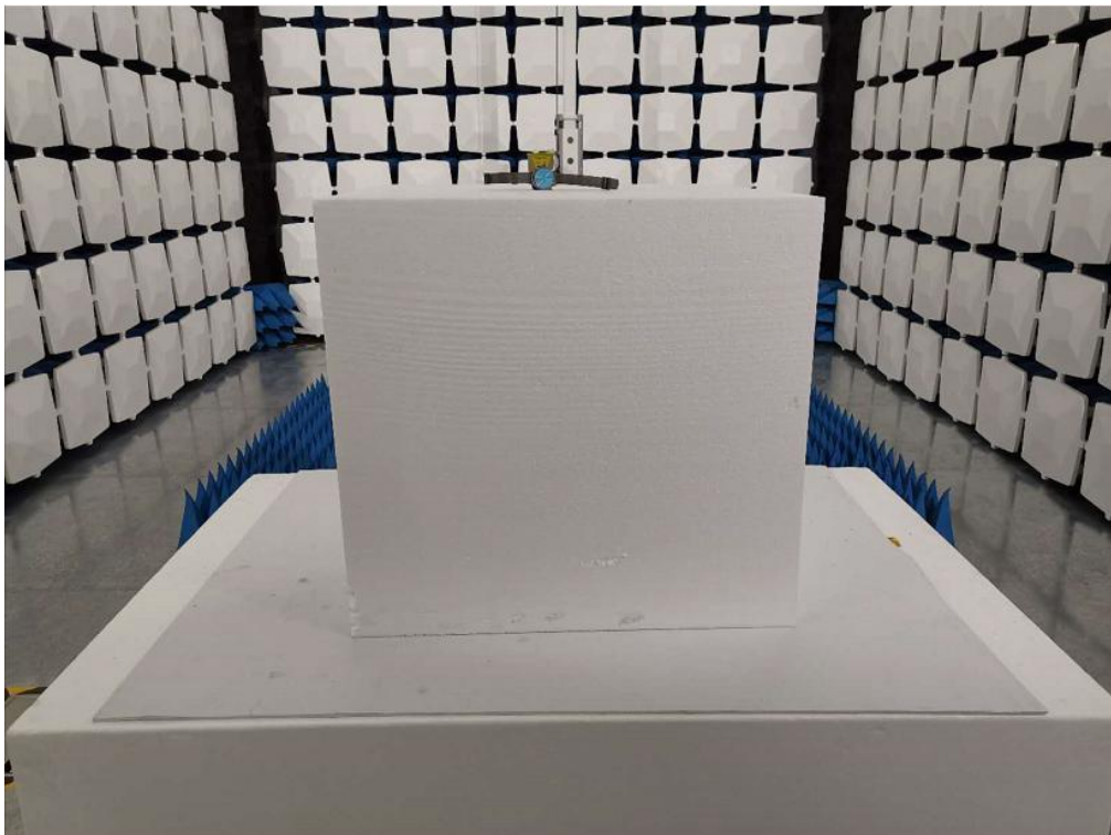
Above 1GHz for radiated emission test setup
