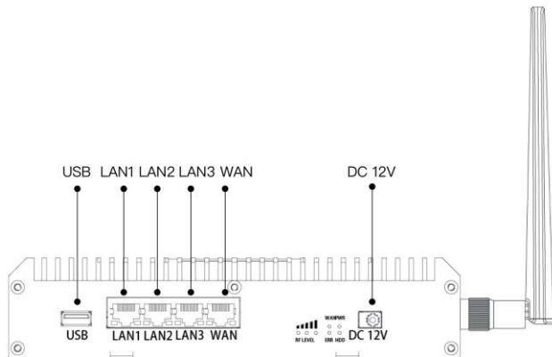
MeshBox Tesla has the following port connections:
