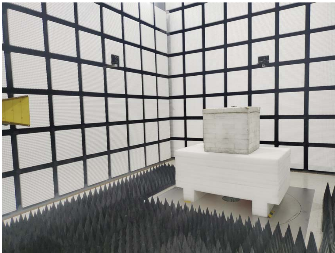
Radiated Emission Above 1GHz
