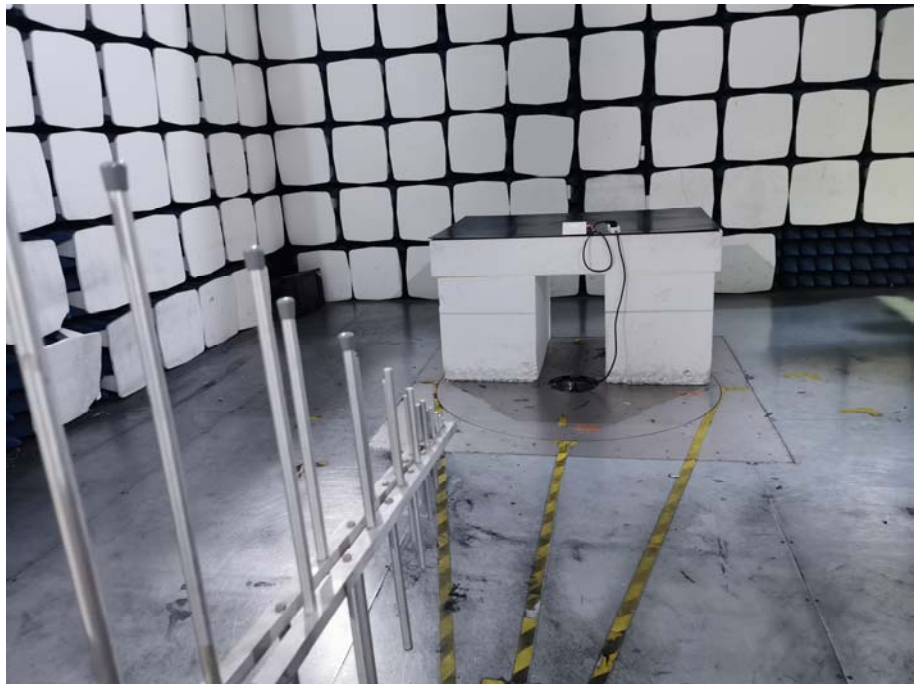
Radiation Emission Test Setup (30MHz to 1GHz)
