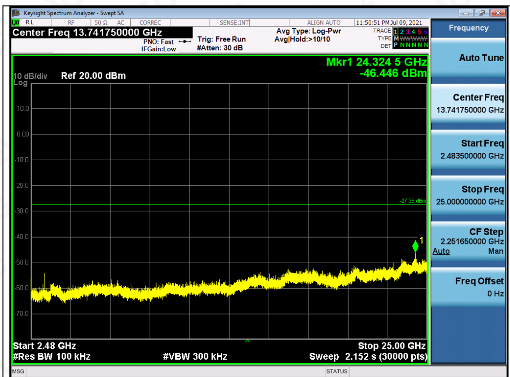
Test_Graph_EDR_ANT1_2441_2Mbps_Higher Band Emissions
