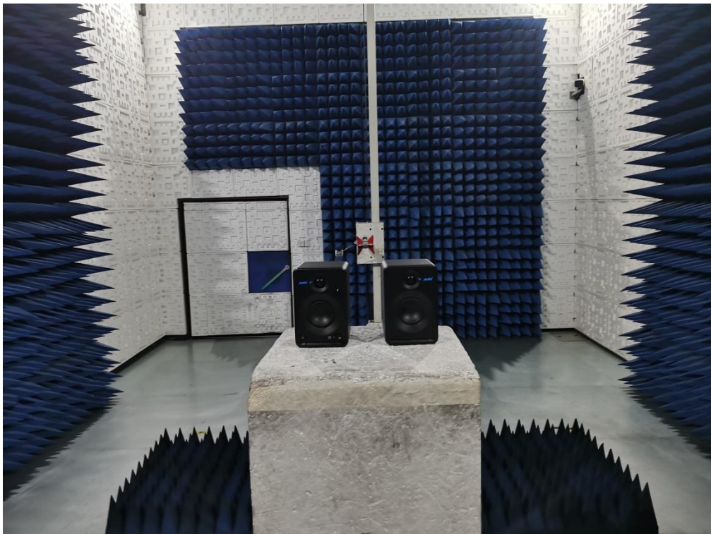
RADIATED EMISSION TEST SETUP ABOVE 1GHz
