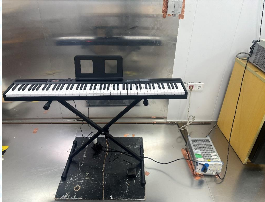
Photo of Setup for Radiated Emission (30MHz~1GHz)
