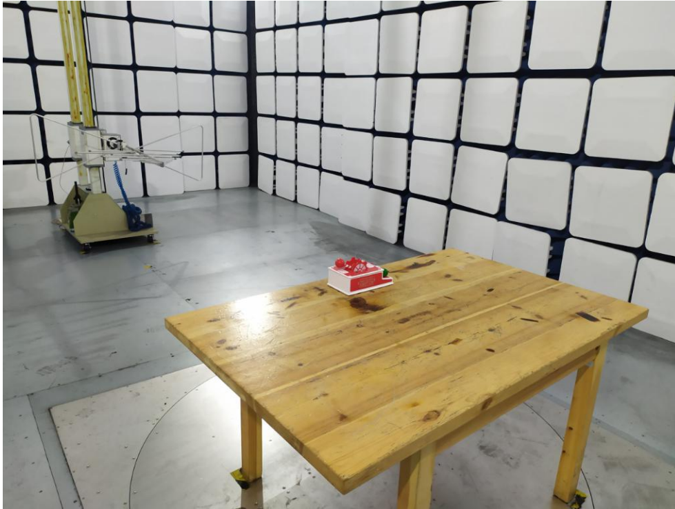
Photo of Radiation Emission Test
