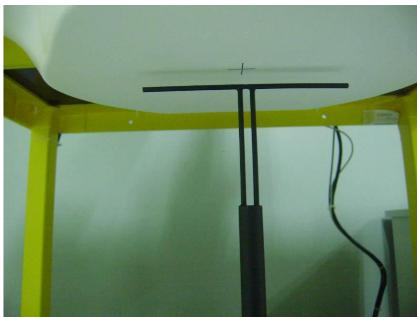
Setup Photo of Dipole Antenna
