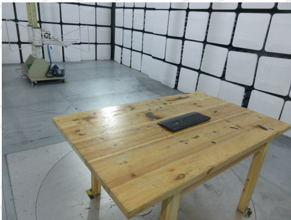
Photo of Radiation Emission Test
