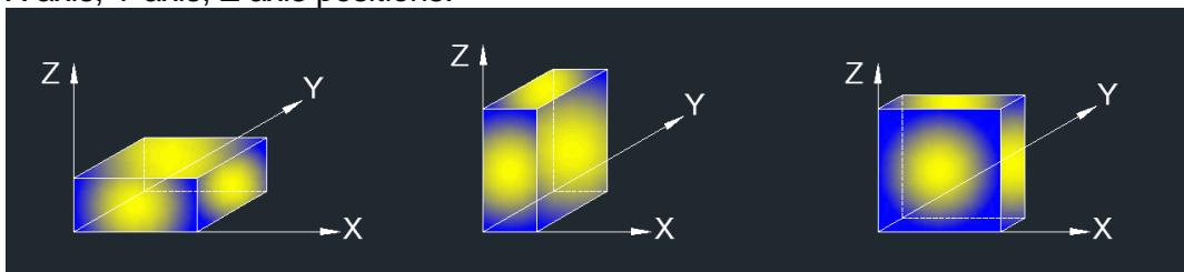
Note: For all radiated test, EUT in each of two orthogonal axis emissions had been tested, but only the worse case (X axis) data recorded in the report.
