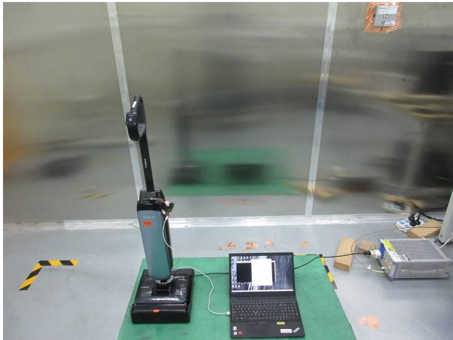
POWERLINE CONDUCTED EMISSIONS MEASUREMENT SETUP
