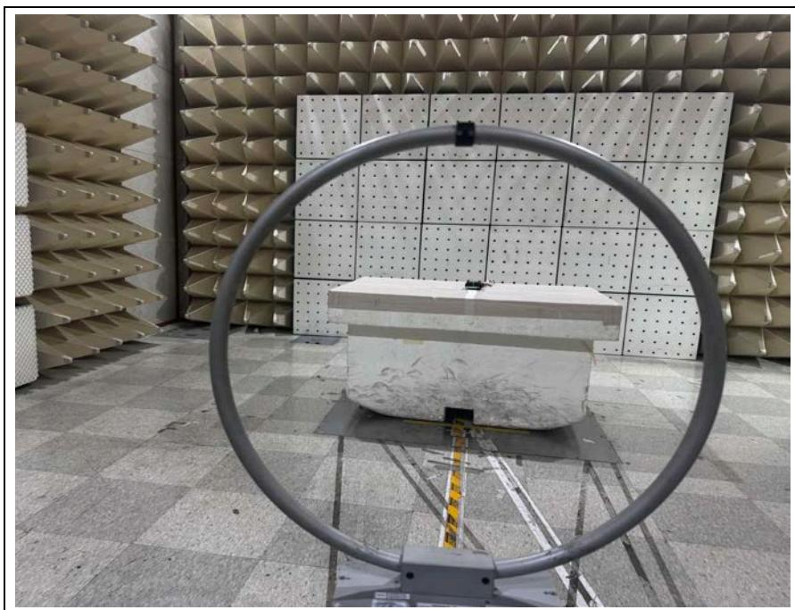
**3. Photo of Radiated Spurious Emission Test (30 MHz ~ 1 000 MHz)**
