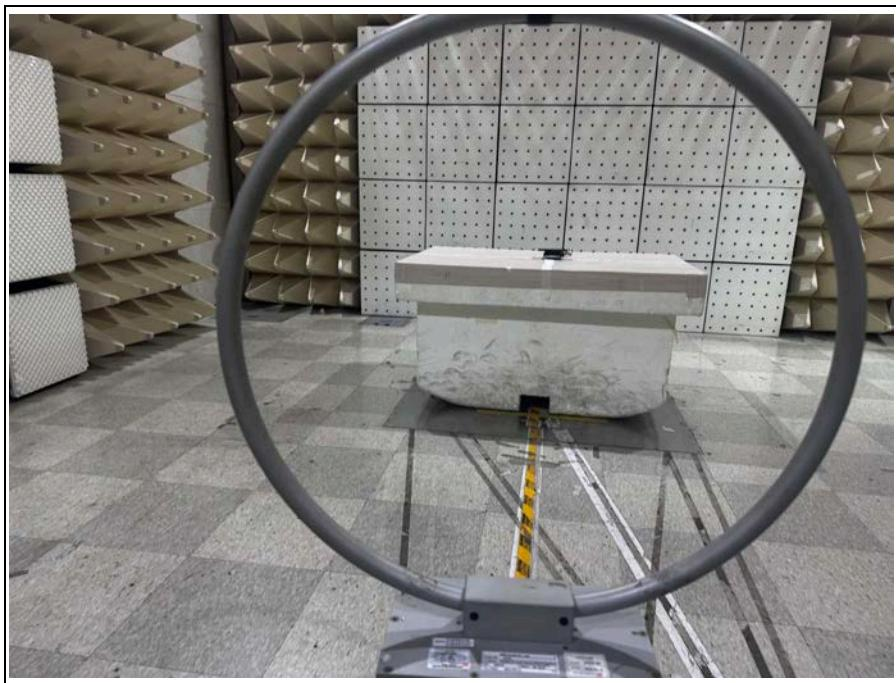
**3. Photo of Radiated Spurious Emission Test (30 MHz ~ 1 000 MHz)**
