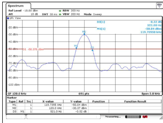
**Test Condition: 10 W Operating mode with client device (1 % battery status of client device)****Ant. 1 (120 kHz)**
