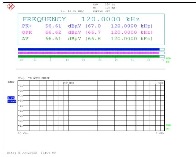
**Test Condition: 10 W Operating mode with client device (1 % battery status of client device)****Ant. 1 (120 kHz)**
