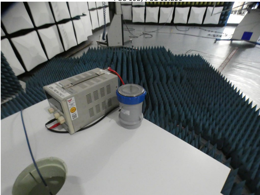
Photo 6: Test setup 1 – 18 GHz, detailed view (SAC)
