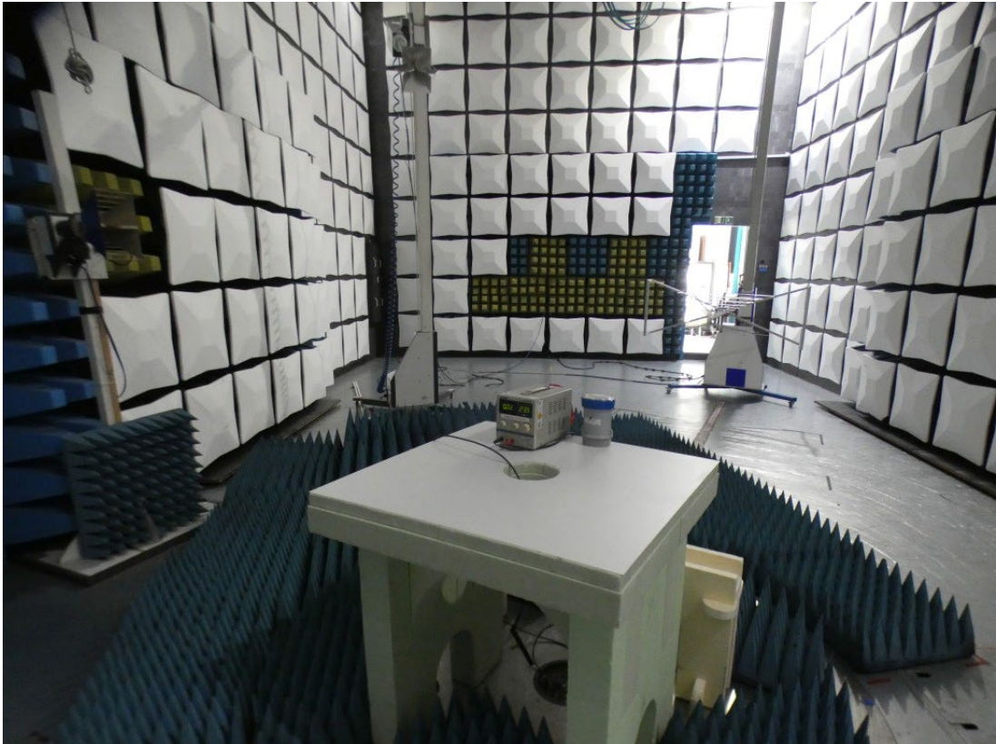
Photo 5: Test setup for radiated emissions measurements 1 – 18 GHz (SAC), FCC 15B, FCC 15.256
