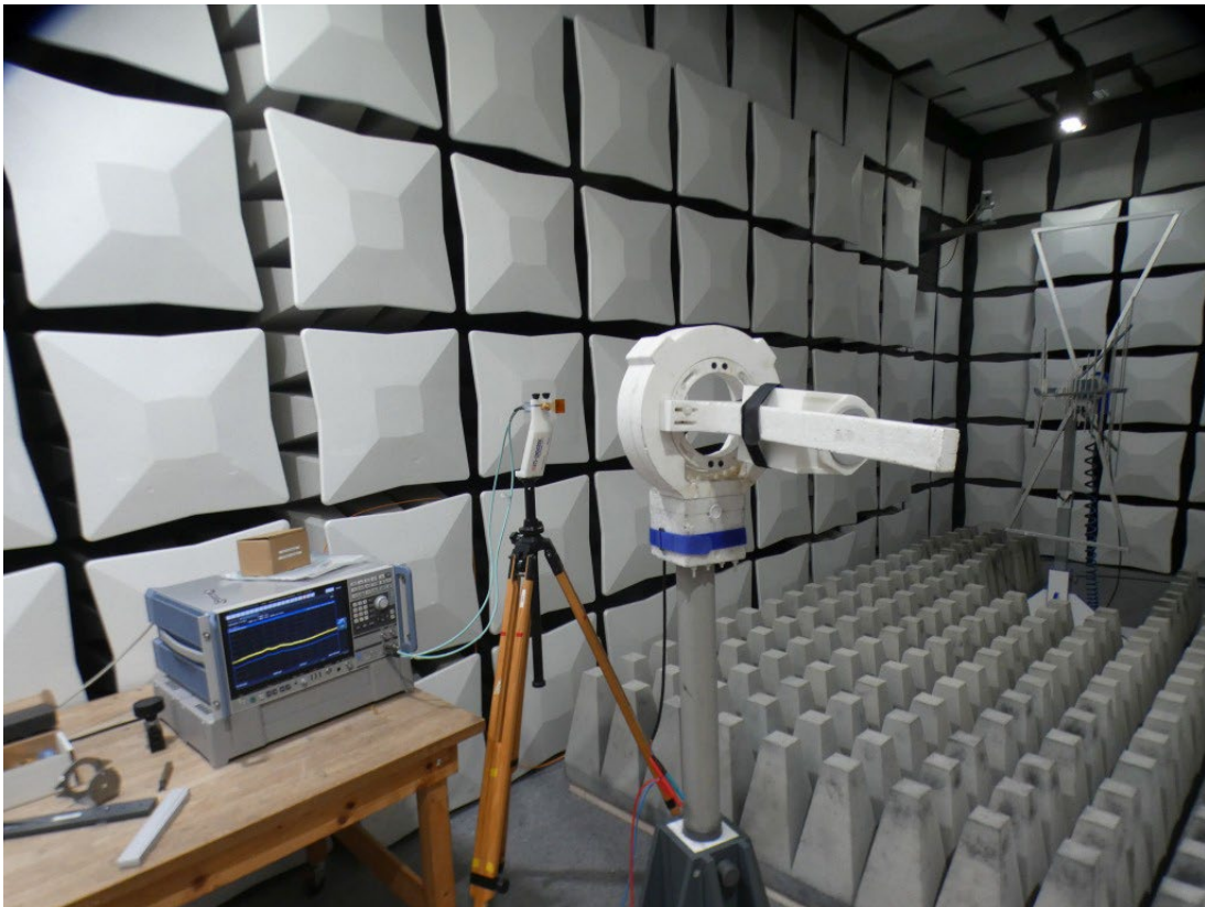
Photo 11: Test setup for radiated emissions measurements 26 - 200 GHz, FCC 15.256 (front side view)
