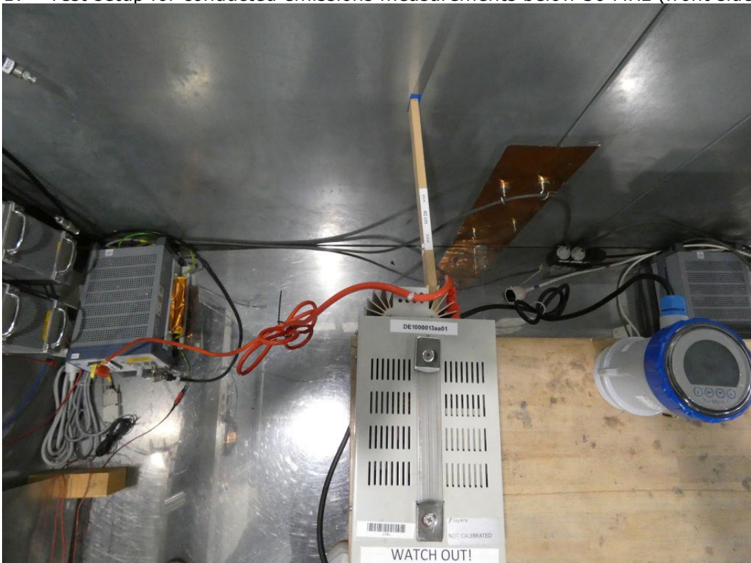
Photo 2: Test setup for conducted emissions measurements below 30 MHz (rear side view)
