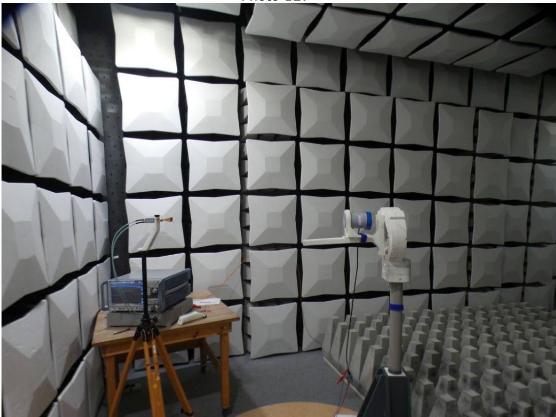
Photo 13: Test setup for radiated antenna pattern measurements 79 GHz (right side view)
