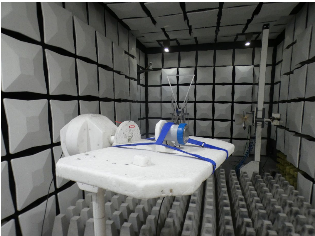
Photo 10: Test setup for radiated emissions measurements 18 - 26 GHz, FCC 15.256 (rear side view)
