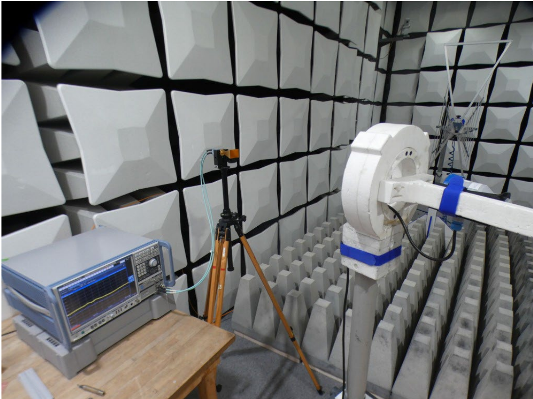
Photo 9: Test setup for radiated emissions measurements 40 - 60 GHz, FCC 15.256 (front side view)
