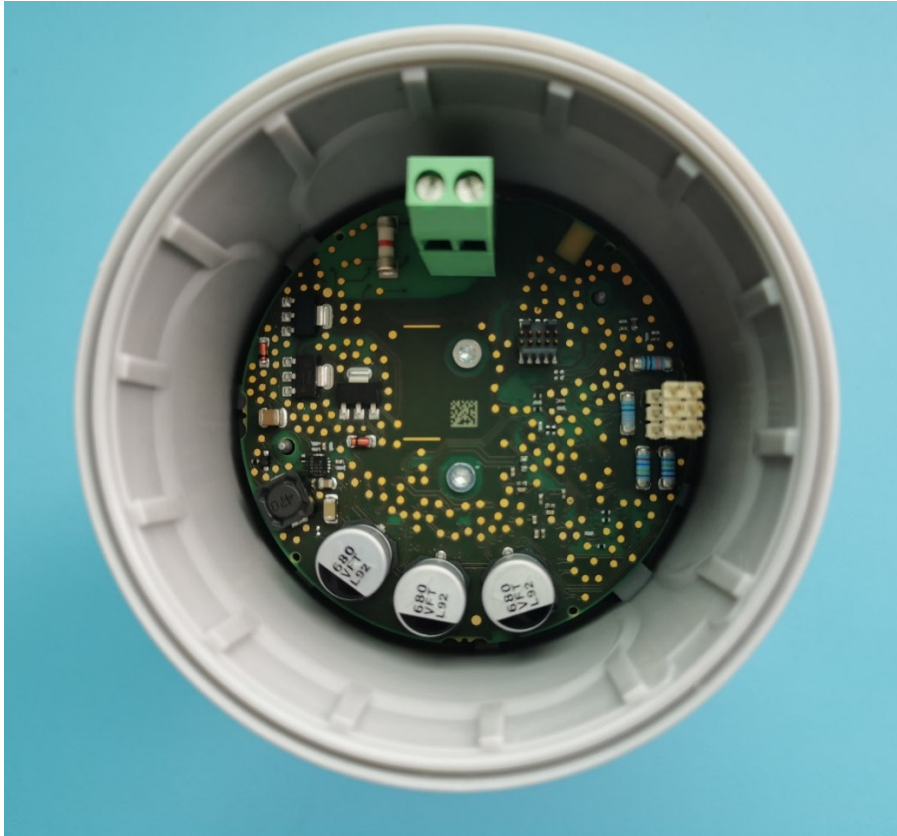
Figure 6: PCB mounted inside the housing
