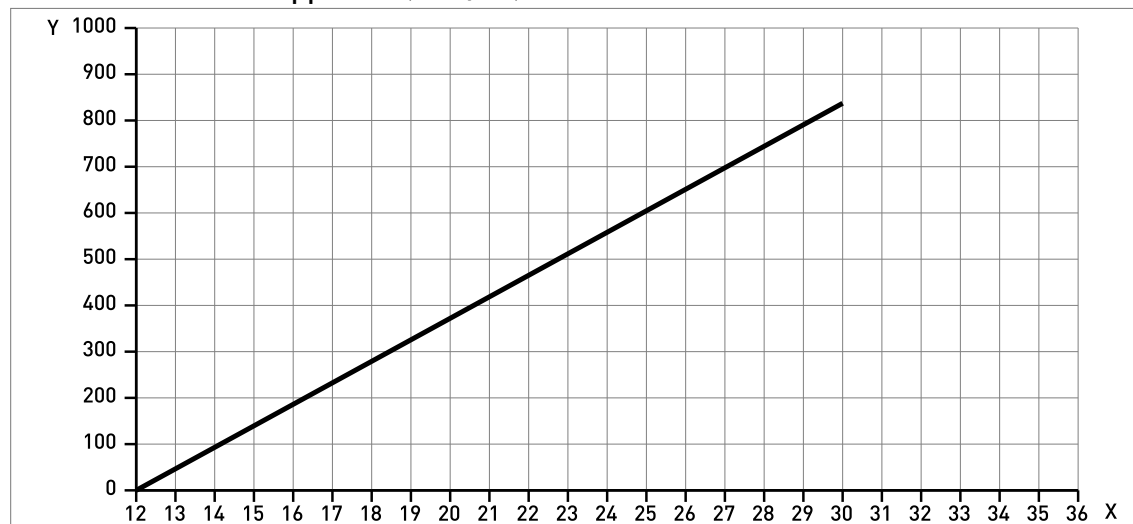
Figure 7-3: Minimum power supply voltage for an output of 22 mA at the terminals (Hazardous Location approval (Ex i / IS))
