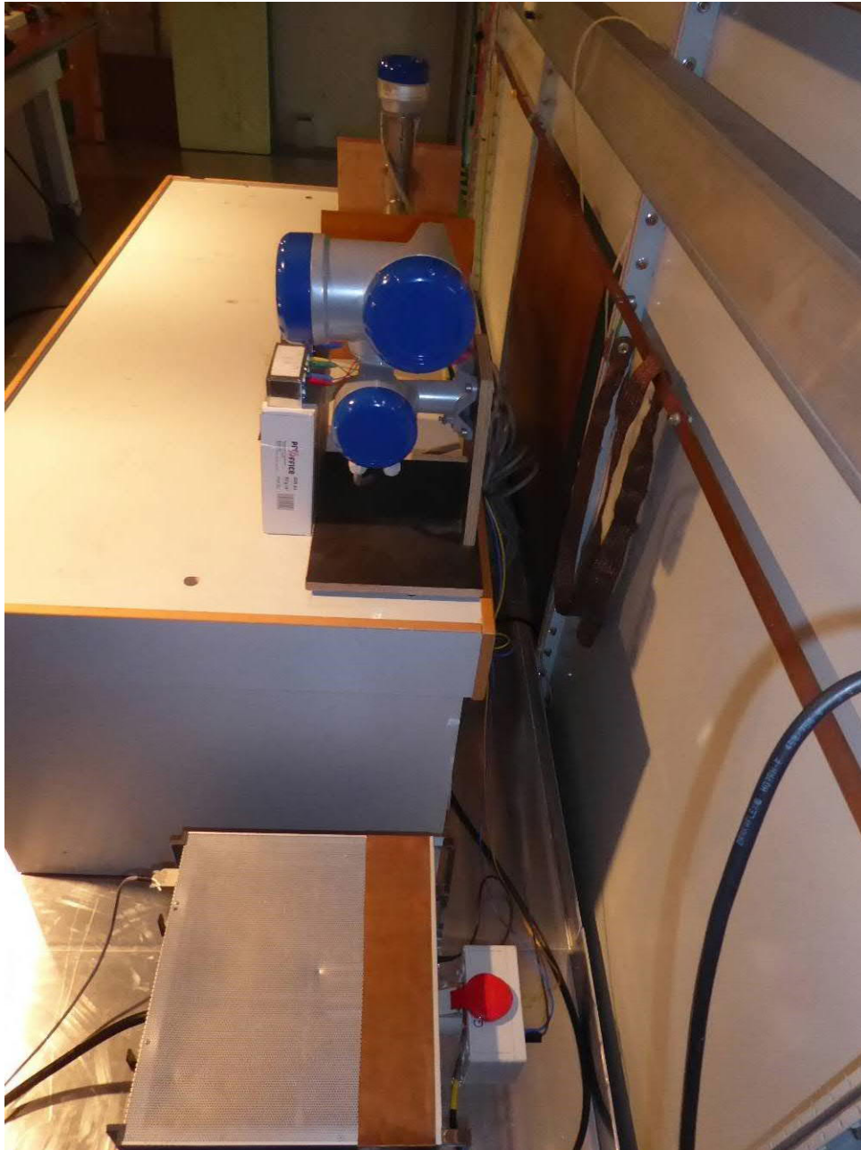
Test setup – power line conducted
