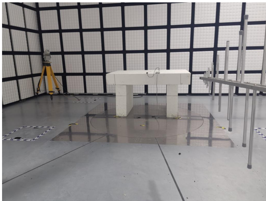
Description: Front view of Radiated Emission Test Setup (Below 1GHz)
