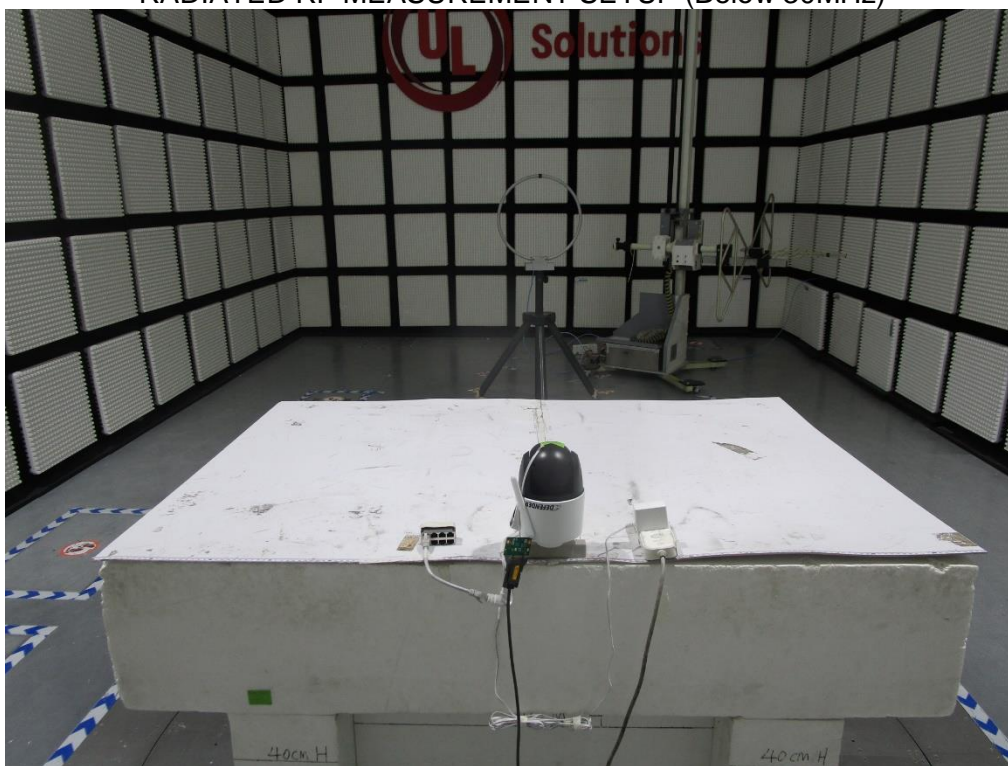
RADIATED RF MEASUREMENT SETUP (Below 30MHz)
