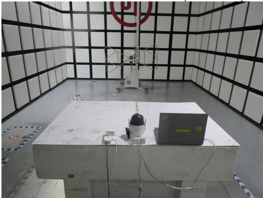
RADIATED RF MEASUREMENT SETUP (Below 30MHz)
