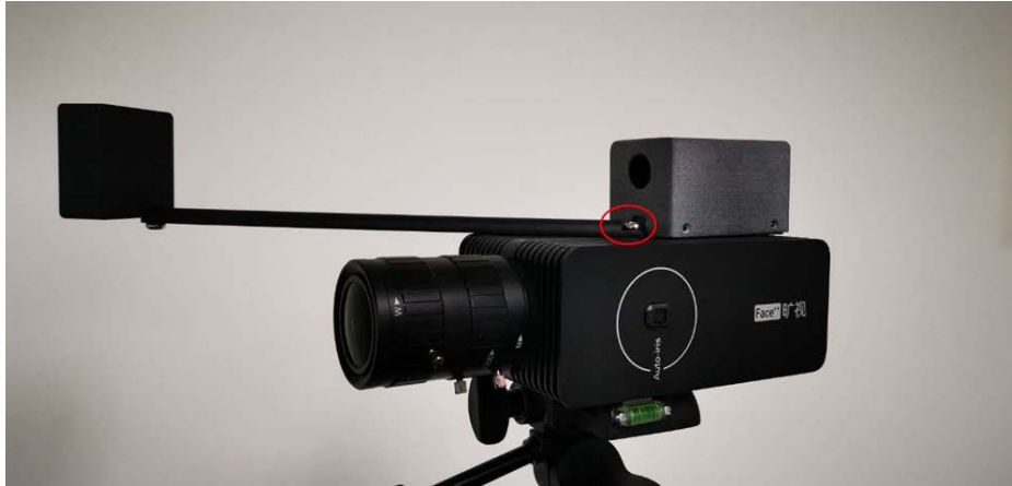
Figure 2-2 Dual-light camera and blackbody assembly
