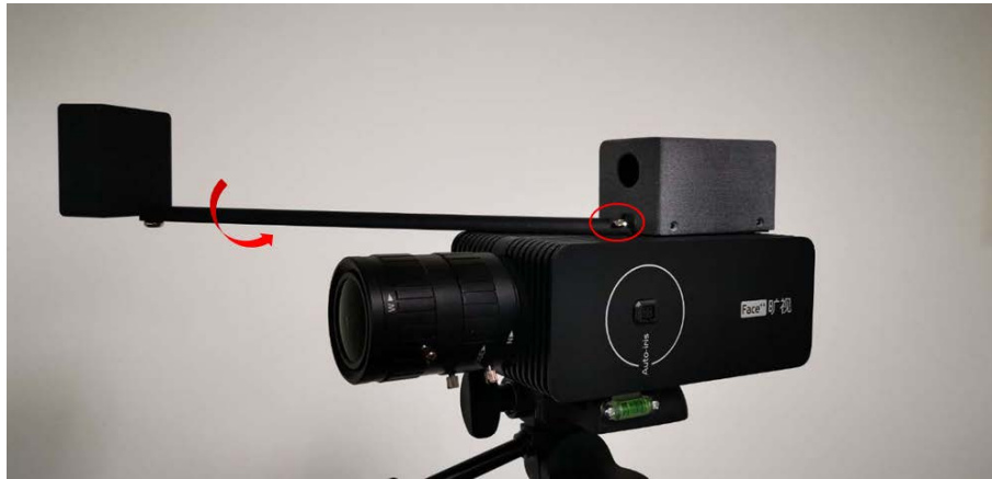
Figure 3-4 Blackbody angle adjustment
