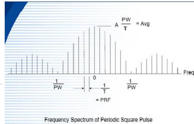
If using spectrum analyzer to measure pulse signal, it have to make sure the RBW use is at least  $2/PW$ .
